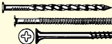
*"The effect of Wolmanized Natural Select™ wood on fasteners is similar to that of CCA treated wood. Hot-dipped fasteners meeting ASTM A-153 are recommended for protection against the moisture often present where treated wood is usually used. For Permanent Wood Foundations, use 304 or 316 stainless steel. Aluminum should not be used in direct contact with this wood."*
